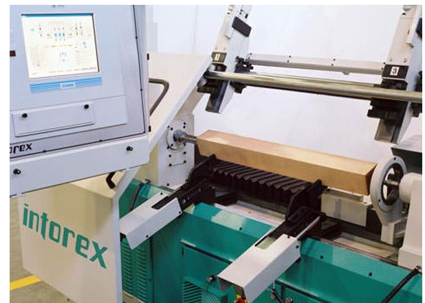
Image 3: Automatic CNC wood lathe ( New Machinery | Intorex CKI Automatic CNC Wood Turning Lathe , no date)
