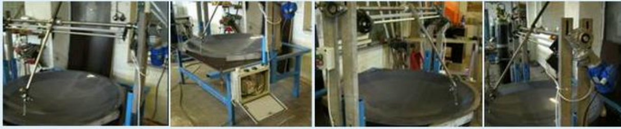
Image 4: The robot and process for laying and gluing thin wire to a spherical surface ( Multitouch hardware. Globe with multitouch Earth application, 2011 )
